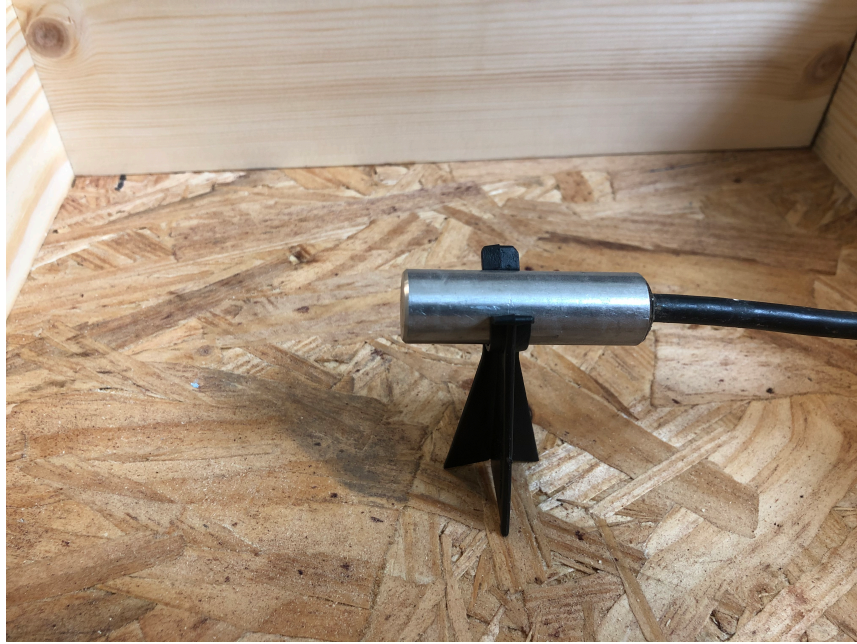
Figure 7 Midpoint Sensor in Concrete Form
