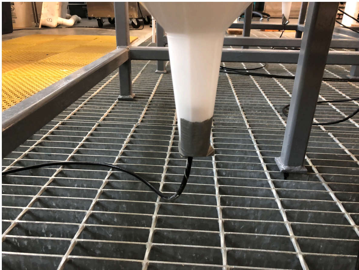
Figure 14 Outflow Temperature Sensor Pervious Concrete
