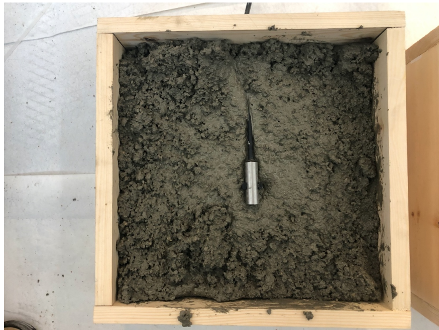
Figure 8 Concrete Temperature Sensor Placement
