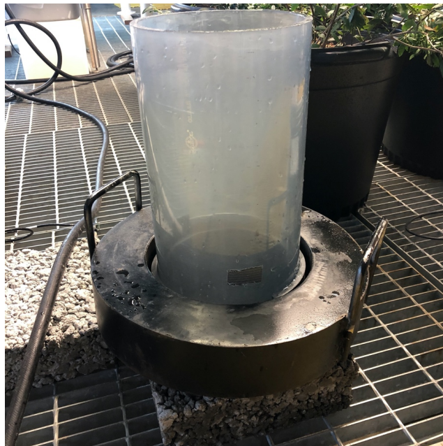
Figure 18 Pervious Concrete Infiltration Rate Testing
