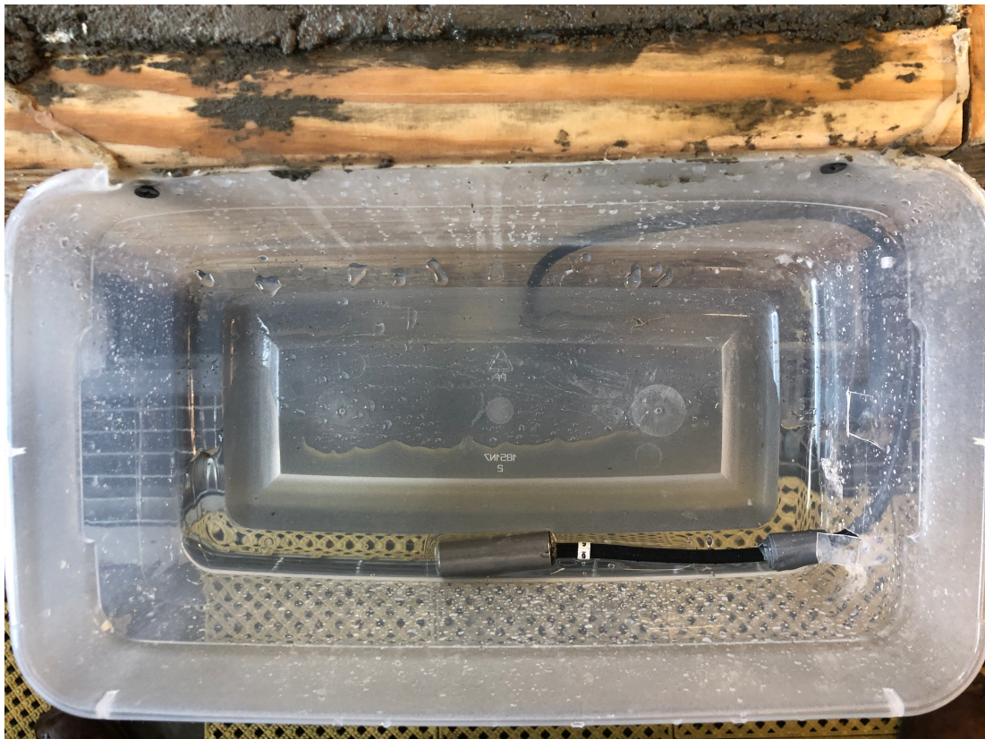
Figure 16 Outflow Temperature Sensor Impervious Concrete
