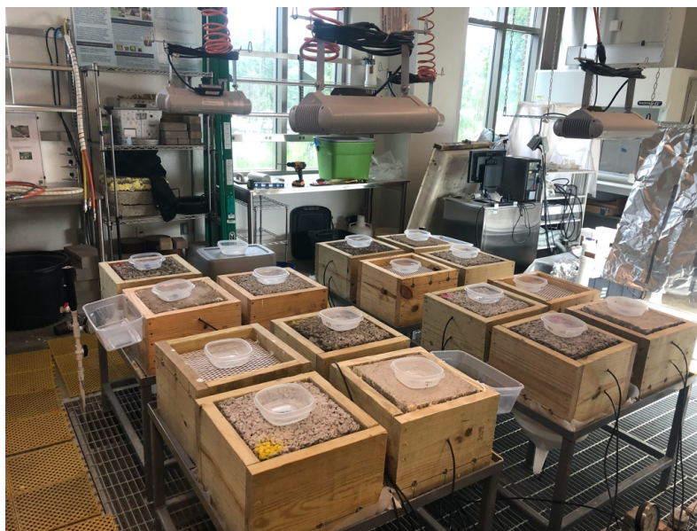
Figure 17 Precipitation Rate and Uniform Distribution Testing
