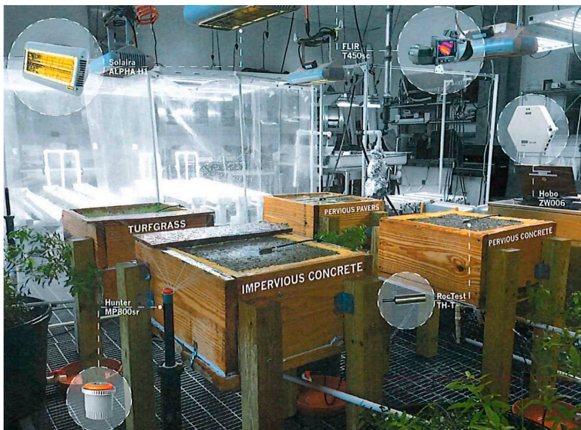
Figure 1. Layout of the Green Infrastructure Laboratory at the Mike Hubbard Center for Advanced Science, Innovation and Commerce (CASIC) Building at Auburn University, Auburn, AL, USA [52].
